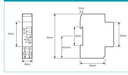
The DRT20 is a variable delay timer to control stairwell lighting.
